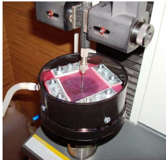
Figure 2. Penetration resistance validation test performed on synthetic cardiac muscle. All of SynDaver Labs' synthetic tissues are validated on the basis of physical tests against actual living tissues.
