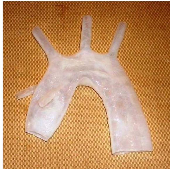
Figure 3. Synthetic human aortic arch with numerous secondary branches. The various branches can be configured in terms of size, angle, and location.
